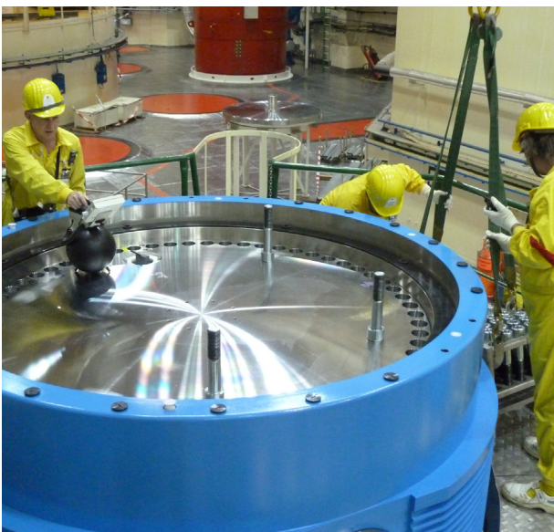
Dukovany NPP spent fuel cask closing ©CEZ
